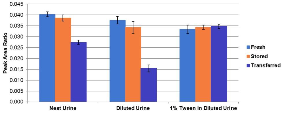
> Non specific binding in urine is common due to the lack of carrier proteins and lipids that can bind analytes. Tween surfactant was added to urine to prevent binding in polyethylene containers. > Loss of AG at low concentrations in DMSO:MeOH (80:20) in glass
